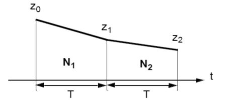
4 equalities, 4 variables:  $z_0$ , c,  $z_1$ ,  $z_2$ , to be solved for:  $z_0$ , c depending on N<sub>1</sub>, N<sub>2</sub>:  $z_1 = z_0 e^{-cN_1}$   $z_2 = z_0 e^{-c(N_1 + N_2)}$ depending on T:  $z_1 = \frac{1}{caT + \frac{1}{Z_0}}$   $z_2 = \frac{1}{ca2T + \frac{1}{Z_0}}$
