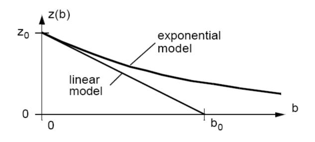
z(b) failure rate, b number of fault locations
