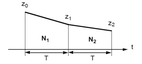
4 equalities, 4 variables:  $z_0$ ,  $b_0$ ,  $z_1$ ,  $z_2$ , to be solved for:  $z_0$ ,  $b_0$ depending on N<sub>1</sub>, N<sub>2</sub>:  $z_1 = z_0 \left(1 - \frac{N_1}{b_0}\right)$   $z_2 = z_0 \left(1 - \frac{N_1 + N_2}{b_0}\right)$
