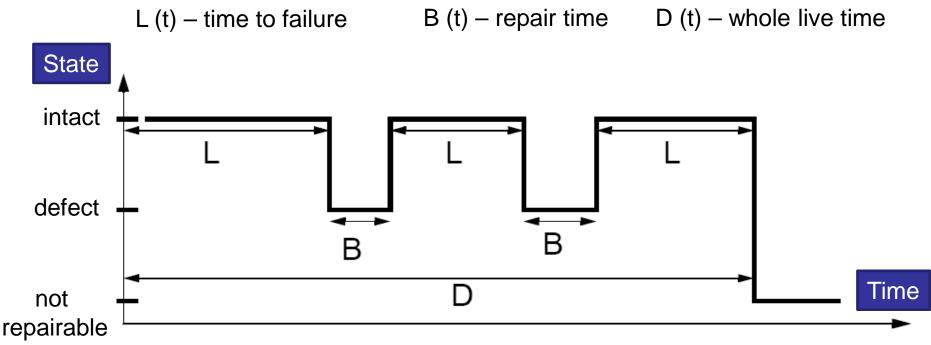
"Time to fault" and "time to failure" have the same meaning. The difference only arise from the layer from which the system is considered.
