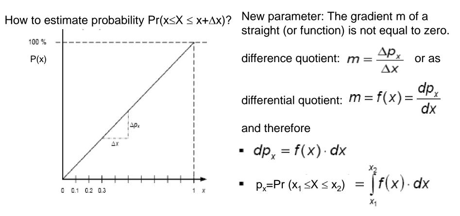
$p_x$  is the probability that values in the interval  $[x_1, x_2]$  are realised. f(x) is the *Density Function*.
