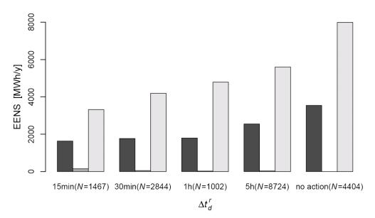
Influence of the operator response time on the EENS due to generation inadequacy (left, black bar), operator action (middle, darkgrey bar) and system splitting (right, light-grey bar) for L=1.37.
