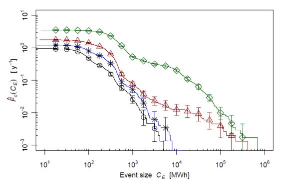
Complementary cumulative blackout frequencies for four different system loading levels L=1.0, 1.1, 1.2 and 1.37 (circles, stars, triangles and diamonds, respectively) without operator intervention. The error bars indicate the 90% confidence interval.
