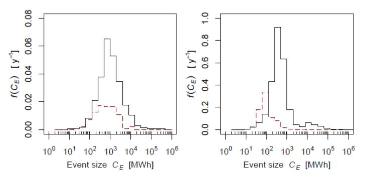
Impact of increasing the system loading from L=1.0 (dashed line) to L=1.37 (continuous line) on the absolute frequencies of blackouts caused by generation inadequacy (left) and system splitting (right).
