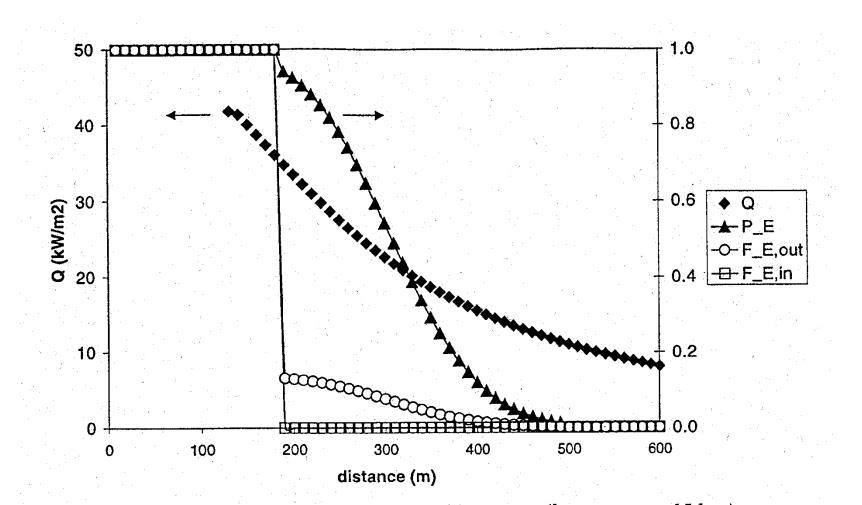
Example calculation of a BLEVE of 100 tonne propane (burst pressure 15 bar). The exposure time is set at the maximum value of 20 s. Indicated are heat radiation, Q, probability of death,  $P_E$ , fraction of people dying outdoors,  $F_{E,out}$ , and fraction of people dying indoors,  $F_{E,in}$ .
