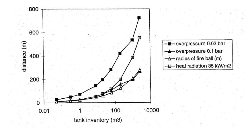
Distances to various effect levels of a BLEVE as a function of tank inventory [TNO98d]. Indicated effect levels are the radius of the fireball, heat radiation equal to  $35 \text{ kW m}^2$  and overpressure levels of 0.1 bar and 0.03 bar.
