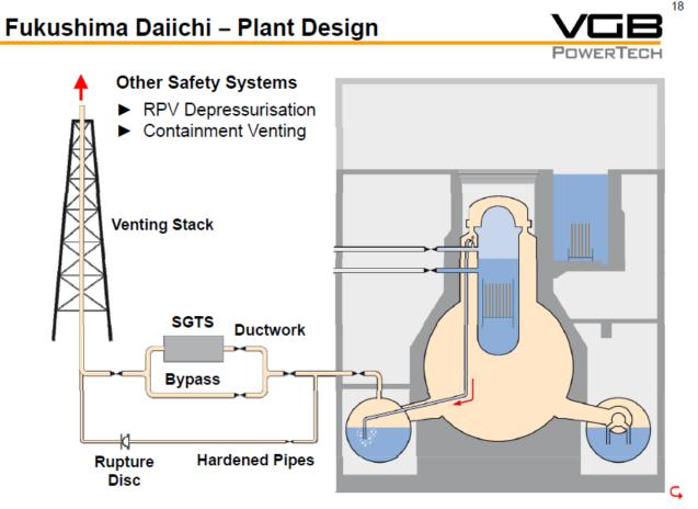
RPV: Reactor Pressure Vessel SGTS: Standby Gas Treatment System
