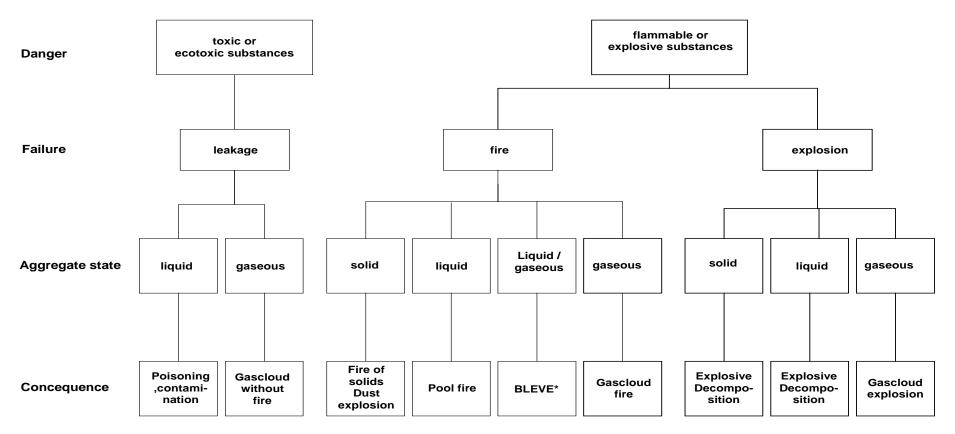
\*BLEVE: Boiling Liquid Expanding Vapour Cloud Explosion
